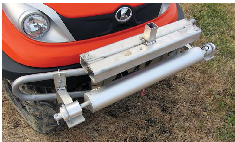
A vehicle-mounted passive gamma-ray sensor.
